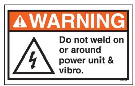
Do *NOT* weld on or around the power unit unless authorized in writing by APE. Doing so will void all warranties and may cause damage to the power unit or vibro.
